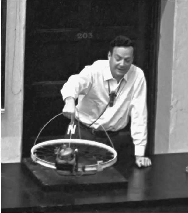
FIGURE 4-9 Feynman demonstrates an artificial gyrocompass.
